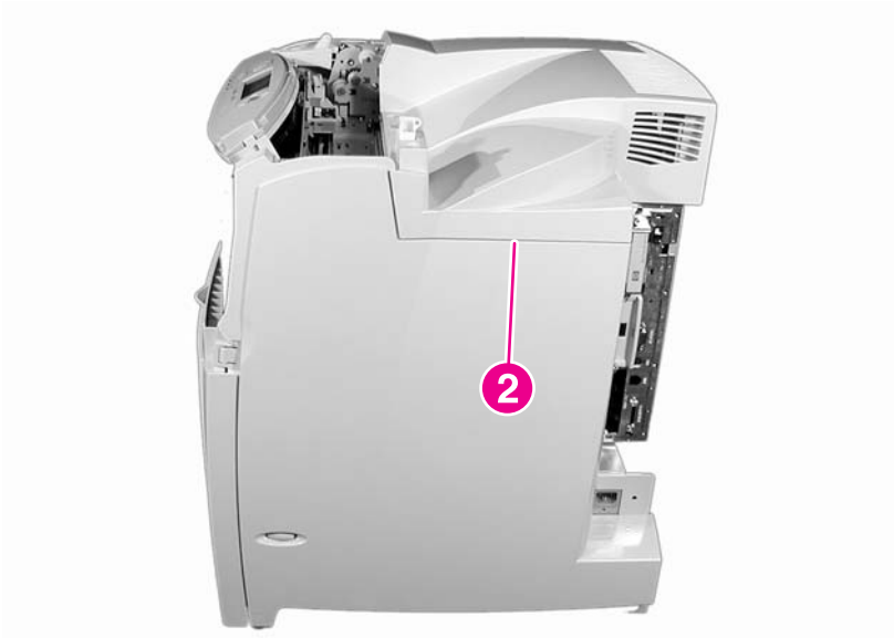
Figure 6-6 Remove the rear top cover (2 of 3)
